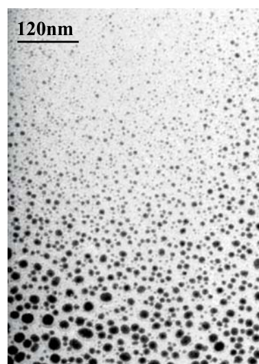
Fig. 5. TEM image of cluster-based nanostructures with number density and size gradient observed at the edge of a shadow area induced by obstructing the cluster beam exposure with a nano-scale object.
